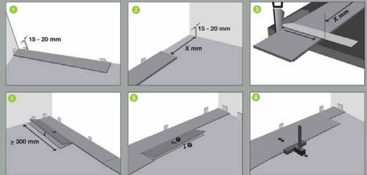
Step 1. The B plate tenon plate A inclined in the fillster locking, and then put it flat.
